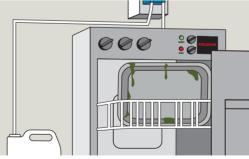
Dispense into automatic machine through an electronic dispenser at a ratio of 2-5ml per litre, at 55-70°C, or in accordance with machine manufacturer's instructions.
